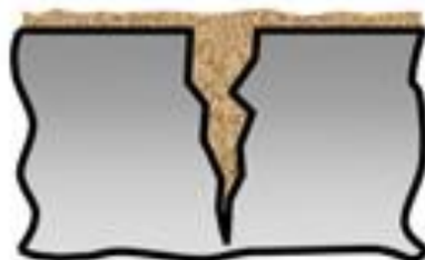
1 Crack filled with dirt
