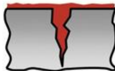
3 Application of penetrant
