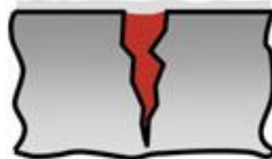
5 Application of developer
