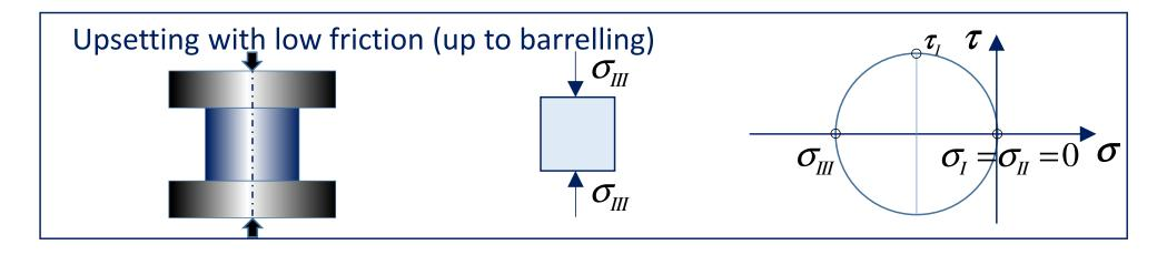
$$-\sigma_{III} = \sigma_f = \frac{F}{A} \quad \text{where } A = \frac{A_o h_o}{h} \quad \text{as} \quad V_o = A_o h_o = A h$$
