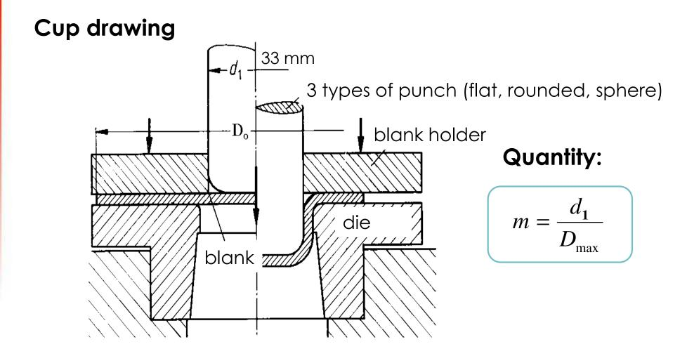
Starting from  $D_o = 58$  mm blank diameter by 2 mm steps till facture (up to max. 74 mm).
