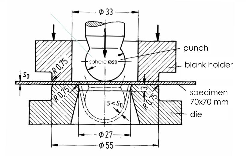
**Quantity:** displacement of the punch from the contact till the crack of the specimen (mm)
