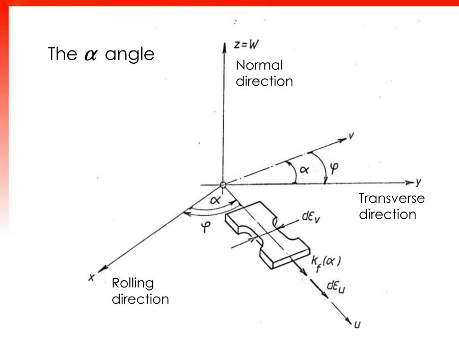
The **Lankford coefficient** is the weighted average of the  $R_{\alpha}$  values measured in the directions 0°, 45° and 90°:
