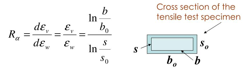
$b_o$  and  $s_o$  are the original, b and s the deformed dimensions. The  $\alpha$  is the angle describing the specimen's orientation relative to the rolling direction of the sheet (see next slide).
